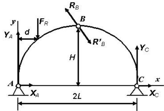
Figure 2. Mechanical model of "wrestling bridge" in the sagittal plane
